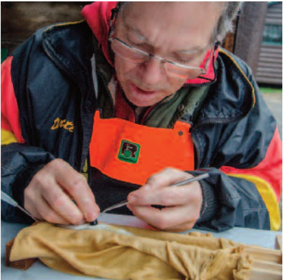
Applying an acoustic transmitter to a salmon smolt.
