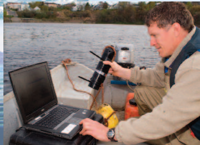
Downloading data from an acoustic receiver. Courtesy of the Atlantic Salmon Federation, Canada.
