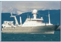
Speed: cruising 13 -14 knots, max 16 knots Endurance: 30 days Bollard pull: max 77 tons, average 60 tons
